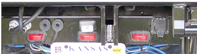
EL-PL-ID WIRE HARNESS FOR (3) CENTER CLEARANCE LIGHTS
